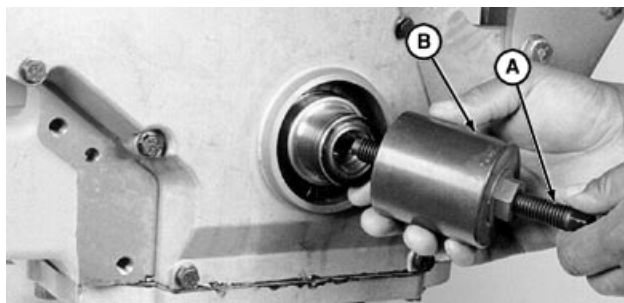
Assembling Puller to Remove Front Wear Sleeve
