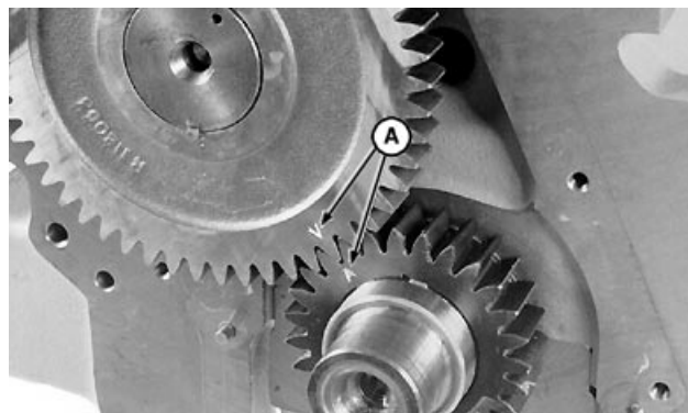
Timing Marks—Camshaft and Crankshaft Gears
