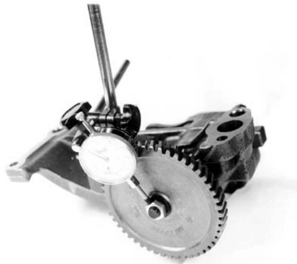
Checking Pump Shaft Side Movement
