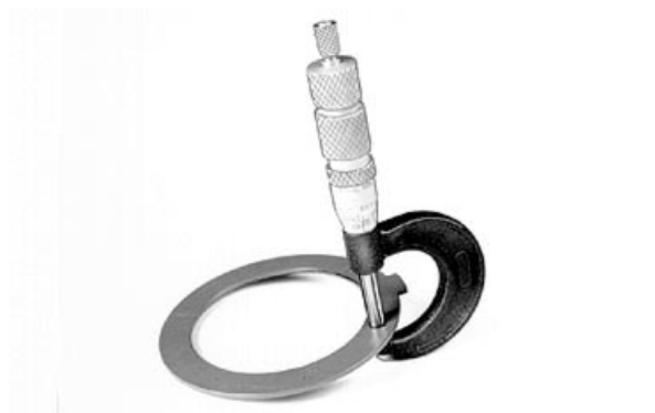
Measuring Camshaft Thrust Washers
