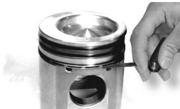
Checking Piston Oil Control Ring Clearance
