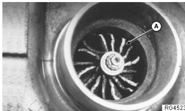
Checking Inlet and Compressor Wheel
