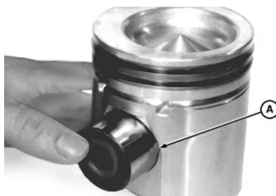
Installing Pin in Piston
