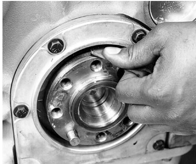
Cleaning Crankshaft Flange
