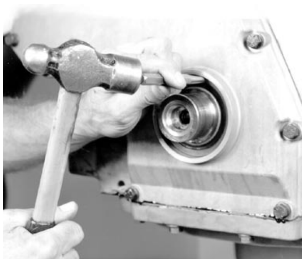
Center Punching Front Oil Seal Casing
