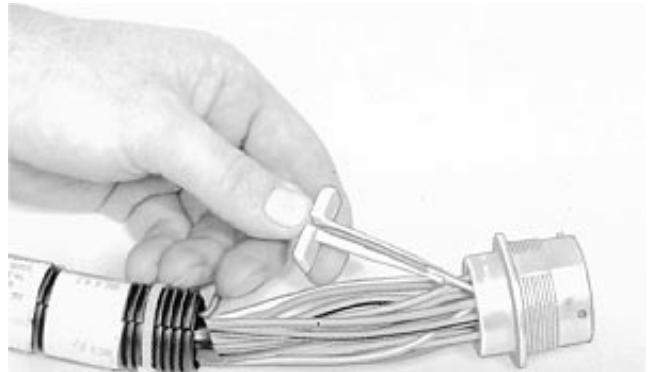
Removing Wire From Connector Body
