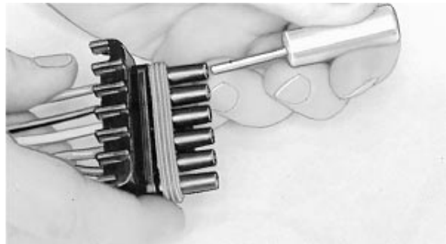
Inserting JDG364 Extraction Tool
