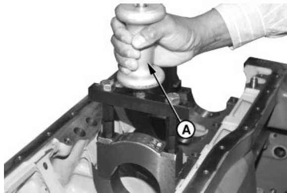
Using Slide Hammer to Loosen Bearing Cap
