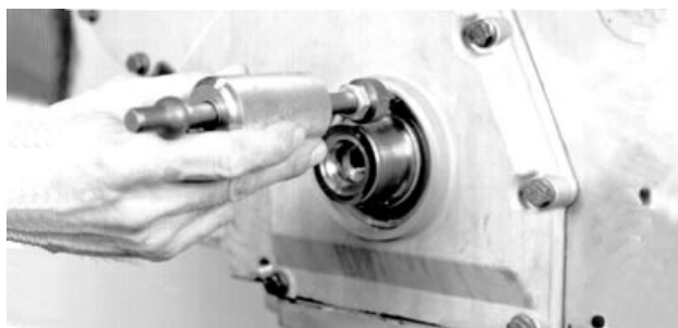
Removing Front Oil Seal
