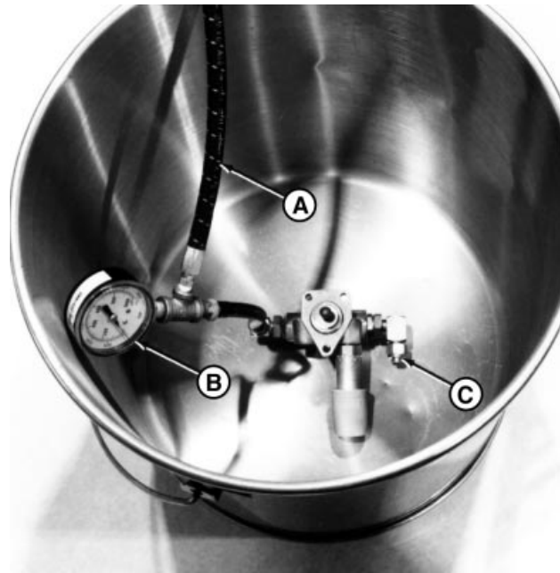
Testing Fuel Supply Pump for Leaks
