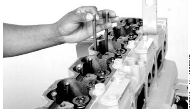
Installing Push Rods and Caps
