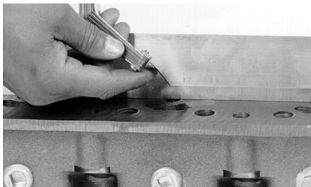
Checking Flatness of Cylinder Head (1)
