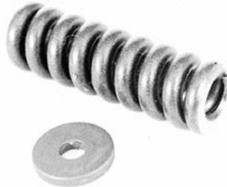
Inspecting Nozzle Spring and Shims
