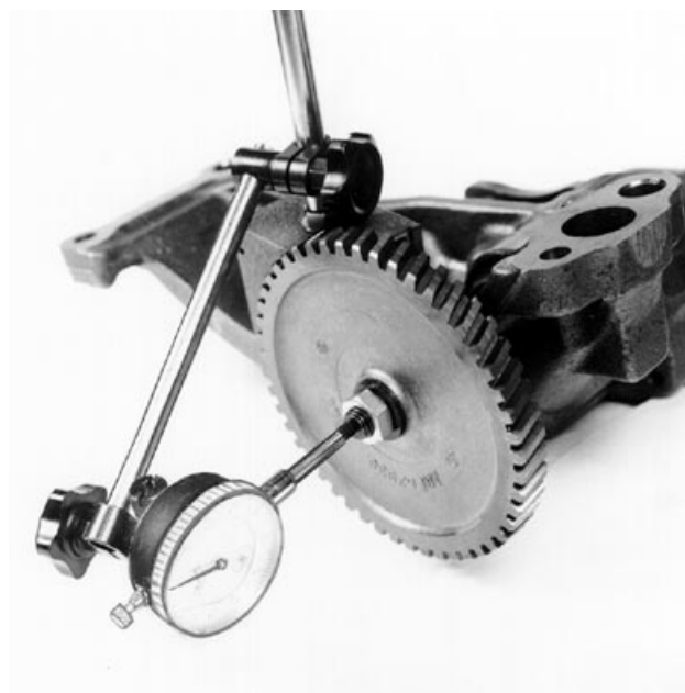
Checking Pump Shaft End Play
