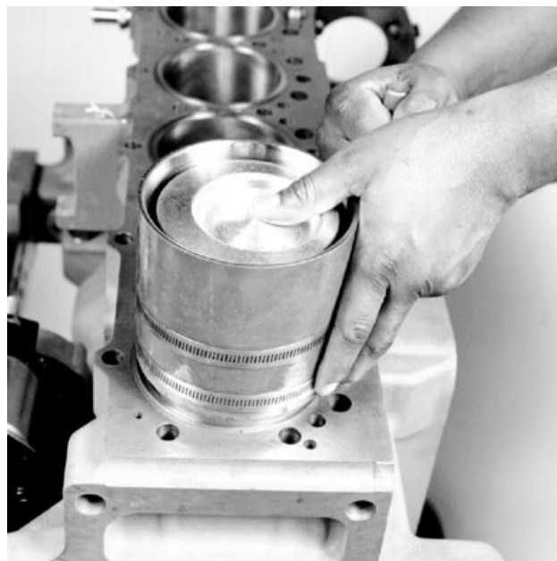
Installing Piston in Cylinder Liners
