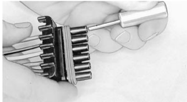
Removing Wire from WEATHER PACK™ Connector
