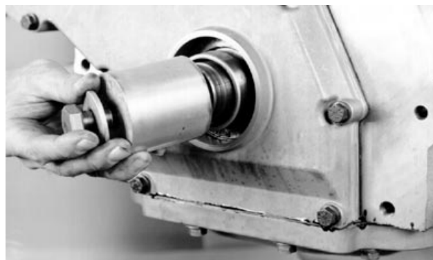
Tool for Installing Front Wear Sleeve
