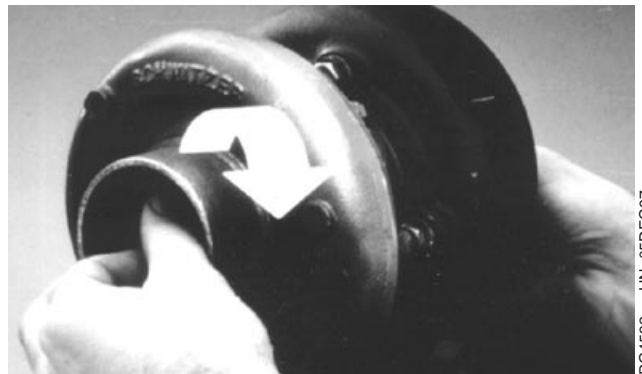
Checking Shaft Rotation and Clearance
