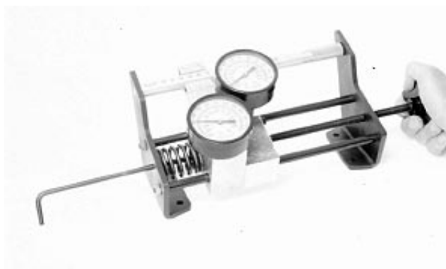
Checking Valve Spring Tension
