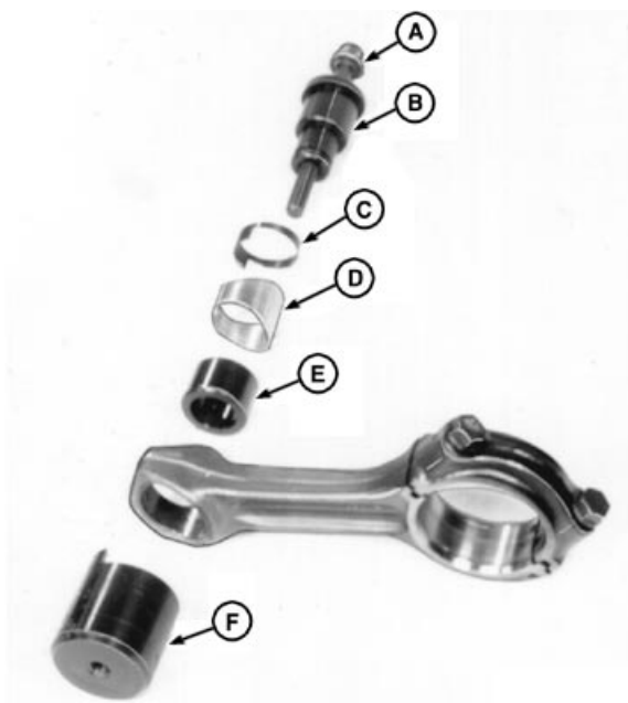
Installing Piston Pin Bushing in Rod
