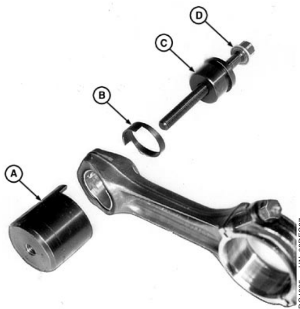
Removing Piston Pin Bushing from Rod
