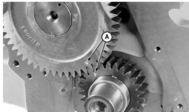
Timing Marks—Camshaft and Crankshaft Gears
