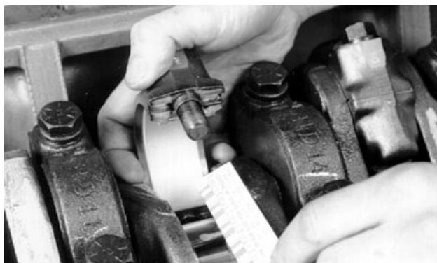
Measuring Rod Bearing-to-Journal Clearance
