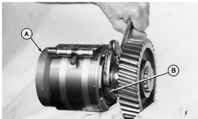
A—Drive Shaft B—Bearing Nut
