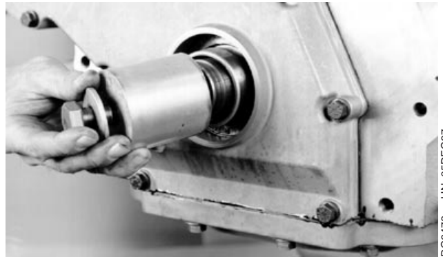
Tool for Installing Front Wear Sleeve
