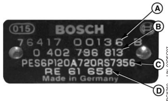
Fuel Injection Pump Identification Plate (Bosch Shown)
