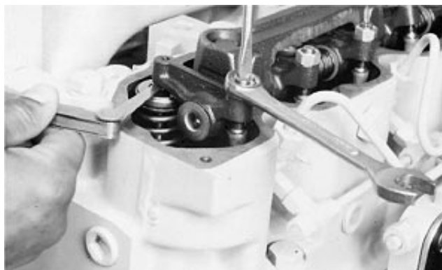
Adjusting Valve Clearance
