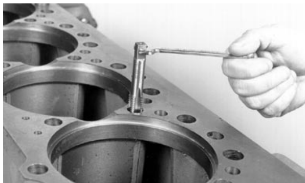
Tap for Head Mounting Holes in Block
