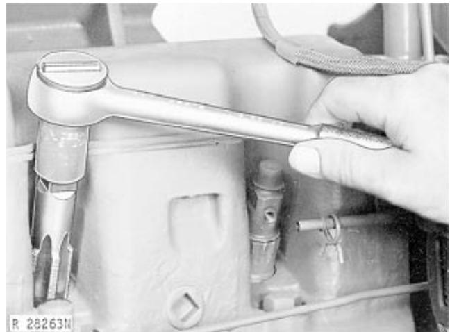
Using Tap to Clean Threads in Nozzle Bores
