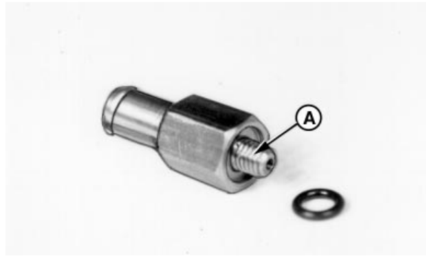
Inspecting Leak-off Connector
