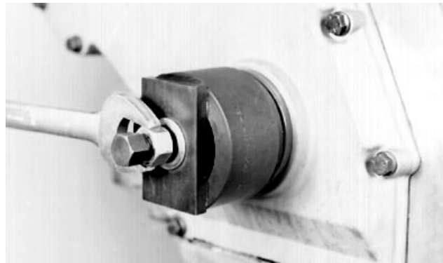
Installing Front Oil Seal
