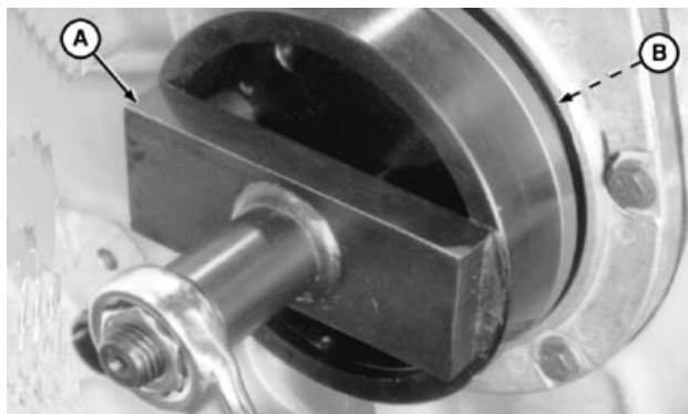
Crankshaft Rear Oil Seal/Wear Sleeve Installed
