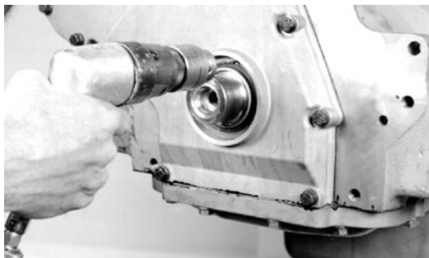
Drilling Hole in Front Oil Seal Casing
