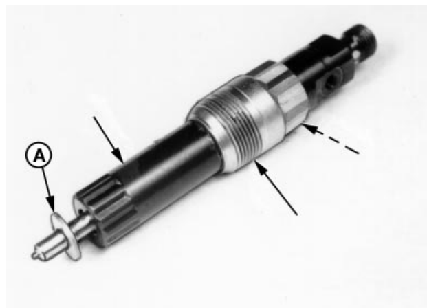
Preparing Nozzle for Installation
