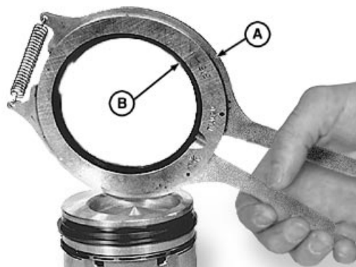
Removing Piston Rings
