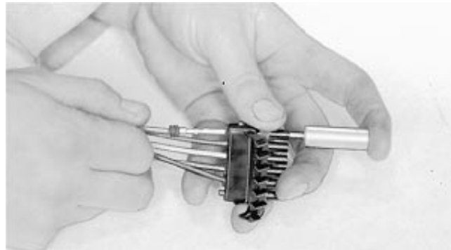
Pulling Wire from Connector Body
