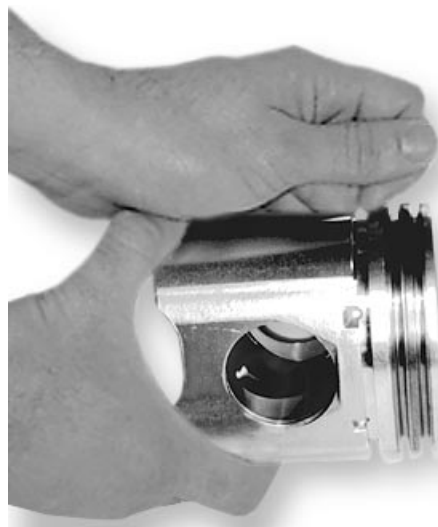
Checking Piston Ring Groove Wear
