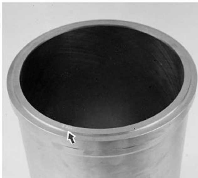
Four-Digit Date Code on Cylinder Liner
