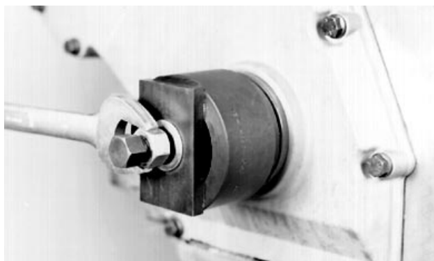
Installing Front Oil Seal
