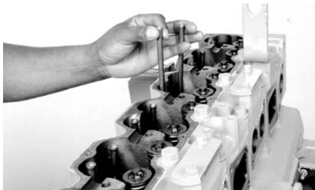
Removing Push Rods
