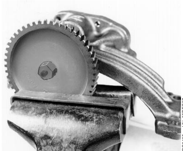
Inspecting Pump Drive Gear
