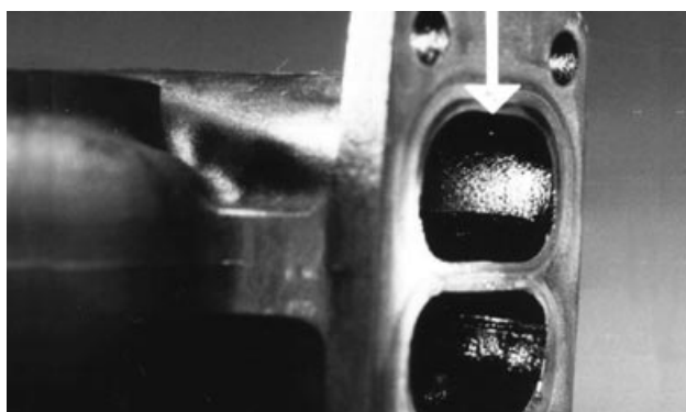
Checking Turbine Housing Inlet Ports
