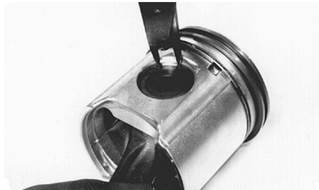
Disassembling Piston and Rod
