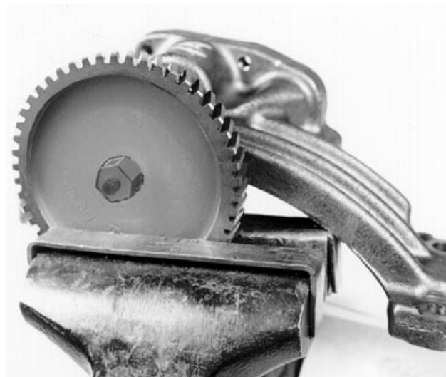
Inspecting Pump Drive Gear
