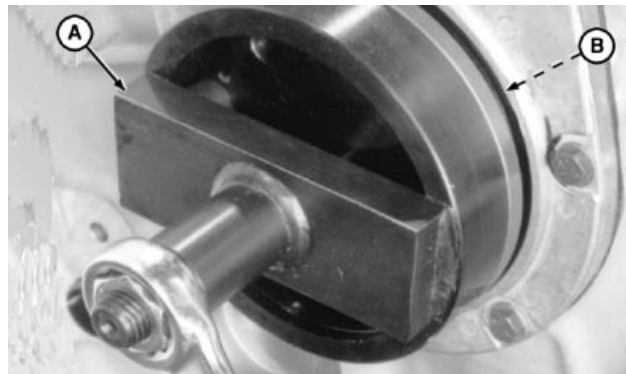
Rear Oil Seal and Wear Sleeve Installed
